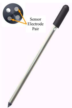
Because EC readings are affected by moisture content, it is important that soil moisture content does not differ significantly between readings. An easy way to achieve this condition is by taking measurements approximately 30 to 60 minutes after an irrigation. This should ensure the soil moisture level has approximately reached field capacity.
