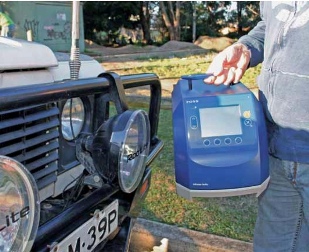
◀ *On farm grain analysis on the move: it takes around three minutes to get a reliable measurement.*
